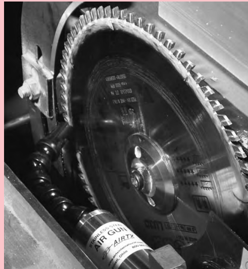
▲ Stainless Steel Air Gun Model 60015
